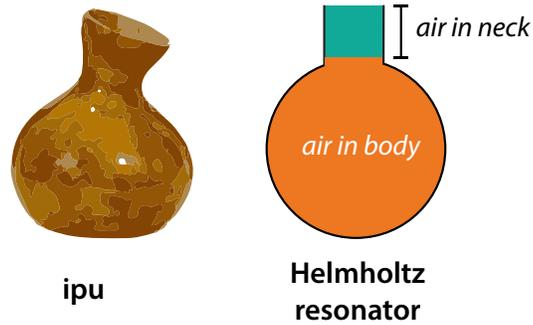
When you hit or blow across a Helmholtz resonator, the air in the neck lightly bounces in and out of the instrument. The air in the neck bounces because the air in the body can be squished and stretched. As the air in the neck bounces, it creates sound waves outside of the instrument.
